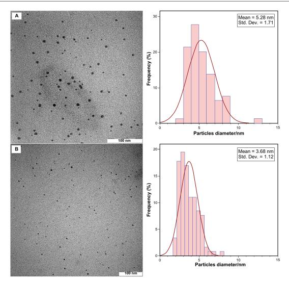
Figure 2 Transmission electron microscopy images and corresponding size distributions of AGG60 (A) and AG60 (B).
