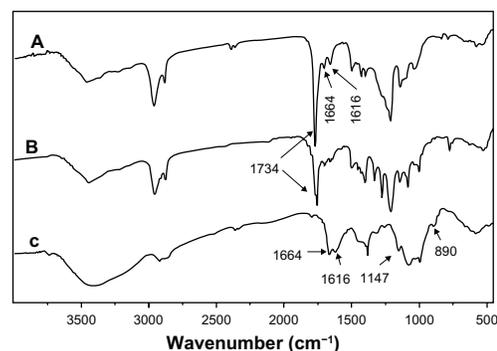
**Figure 2** Fourier-transform infrared spectra of CS-PCL (A), PCL (B), and CS (C). **Abbreviations:** CS, chitosan; CS-PCL, cationic chitosan-graft-poly ( $\epsilon$ -caprolactone); PCL, polycaprolactone.
