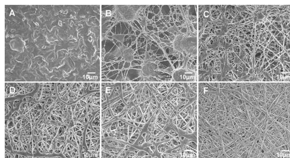
**Figure 3** Scanning electron microscopy images of electrospun nanofibrous scaffolds prepared from different CS-PCL/PCL weight ratios: CS-PCL (A), CS-PCL/PCL (80/20) (B), CS-PCL/PCL (60/40) (C), CS-PCL/PCL (40/60) (D), CS-PCL/PCL (20/80) (E), and PCL (F).
