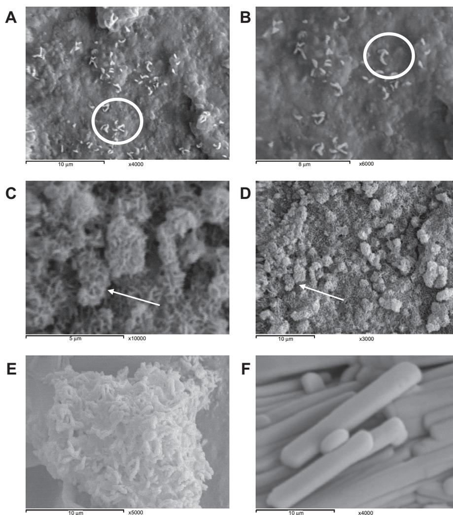
**Figure 1** Nanoparticles (A), close up of theophylline nanoparticles (B), theophylline controlled agglomerates (C), close up of theophylline controlled agglomerates (D), aggregation of theophylline nanoparticles upon using high concentration of NaCl (E), and theophylline powder without processing (F). Note the circles that showing the mechanism of self-assembly of nanorods on a copper grid. The arrows show fluffy spherical nanorods of the controlled agglomerates.
