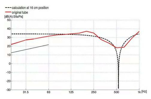
Figure 3 The measured and calculated pulmonary sound pressure levels of the cylindrical tube stethoscope.
