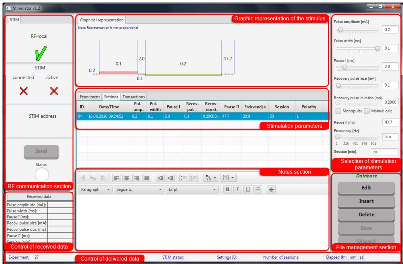
**Figure 2** Software program graphic user interface (GUI) used for the control of the stimulation parameters. The specific sections of the GUI interface are marked with red squares and additionally explained. The right side of the GUI contains sliders that are used for defining the stimulation parameter.
