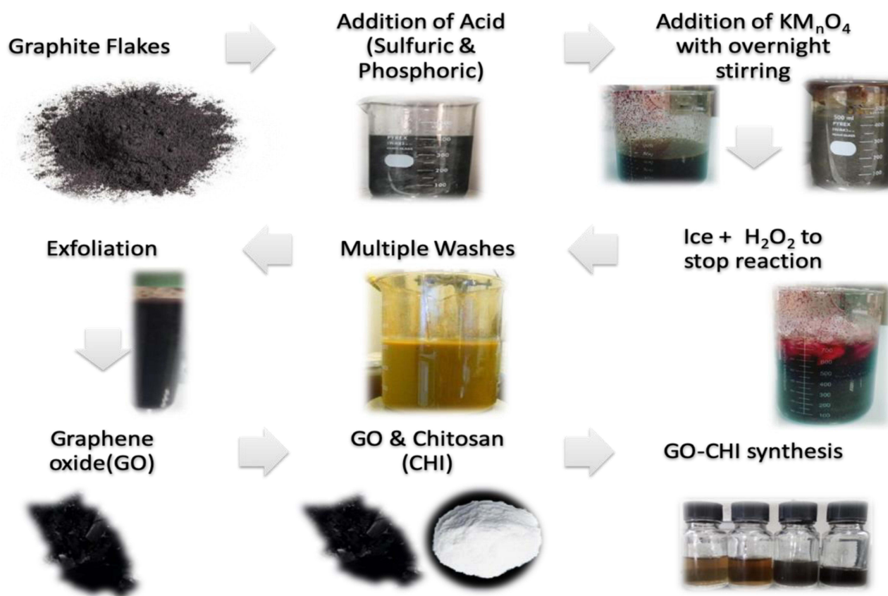
Figure 1 Step-wise synthesis of GO by improved Hummer's method and GO-CHI nanocomposite.
