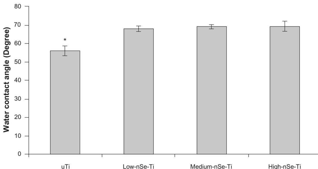
**Figure 2** Water contact angles on the uncoated and Se-coated Ti substrates. Contact angles increased on the substrates coated with selenium nanoclusters. **Notes:** Data = mean  $\pm$  SEM; N = 3; \*P < 0.05 compared to all the coated substrates. There was no significant difference among the contact angles on the coated substrates. **Abbreviations:** Se, selenium; SEM, standard error of mean; Ti, titanium.
