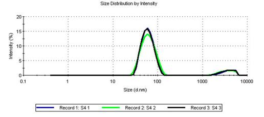
Figure I Particle size distribution of the formed titanium dioxide nanoparticles measured by dynamic light scattering analysis.
