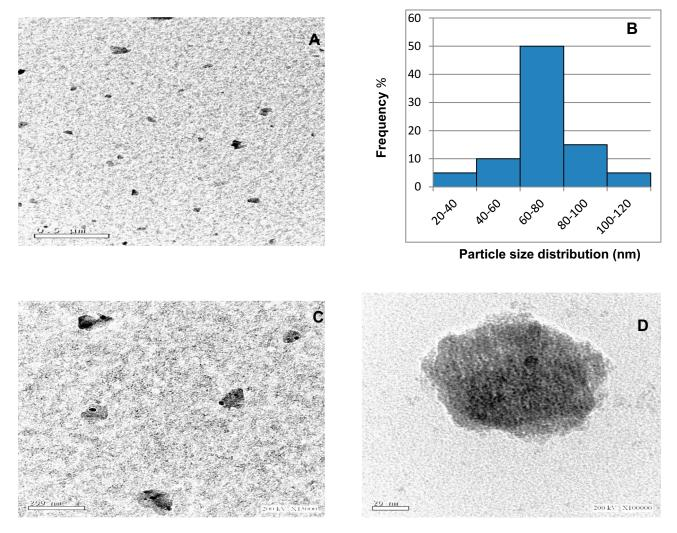
Figure 2 High-resolution transmission electron microscopy images at different magnifications (A: ×5000, C: ×15,000 D: ×100,000) showing the prepared titanium dioxide nanoparticles as spherical shape with an irregular edges. (B) Particle size distribution of it.
