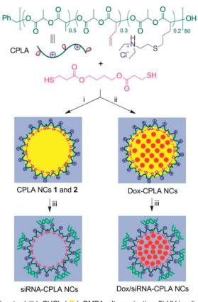
i: 1) water ( ■ ), CHCl<sub>3</sub> ( ■ ), DMPA, ultrasonication; 2) UV irradiation ii: same as i, except Dox ( ● ) addition and extraction
