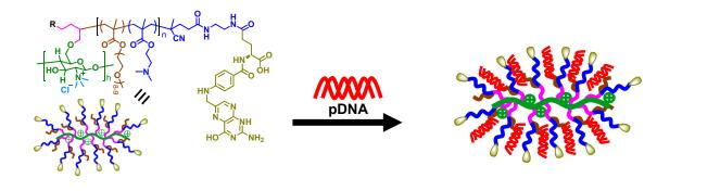
Figure 6 Preparation of TCS-g-poly(PEGMA-co-DMAEMA)-FA/pDNA polyplexes.
