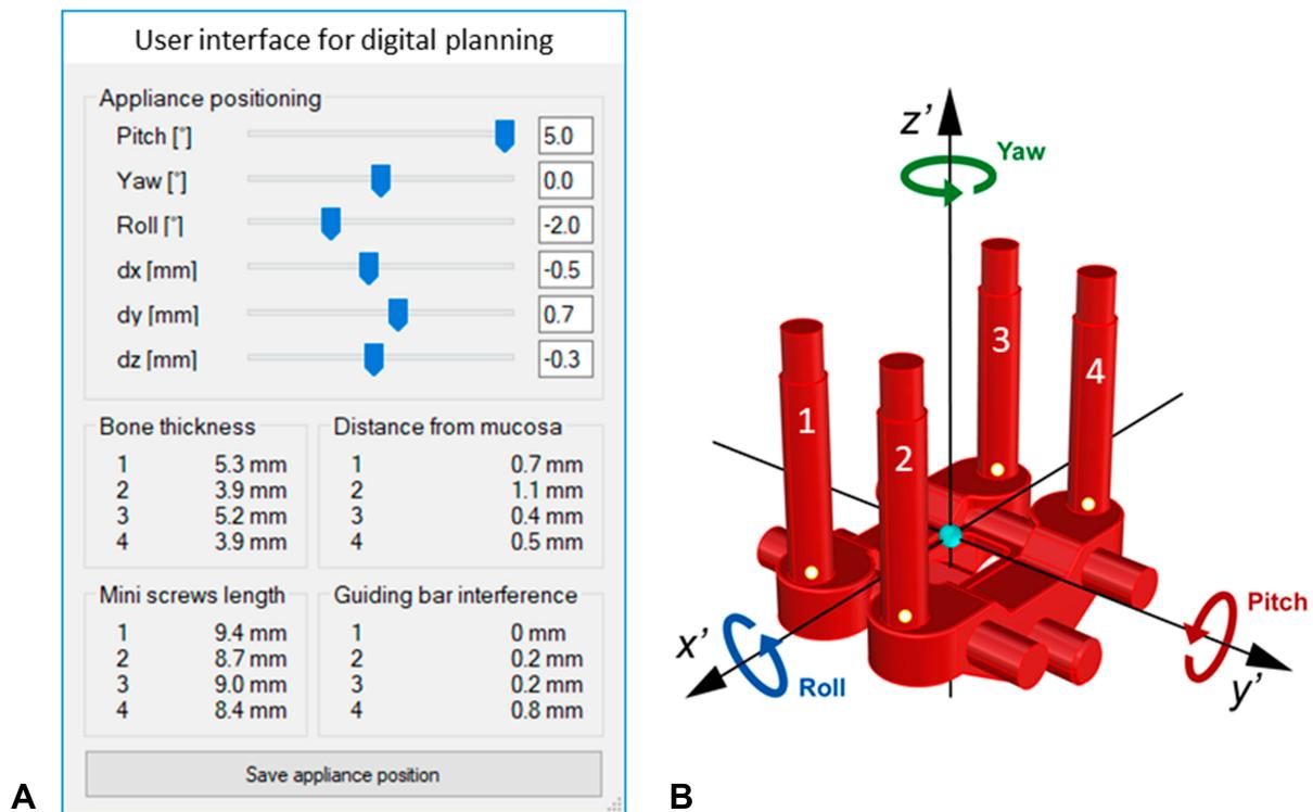
**Figure 6 (A)** User interface developed with Rhinoceros software, with which the inclination (Yaw, Pitch, and Roll) and position (dx, dy, dz) of MSE appliance can be changed to optimize the bone thickness (BT) at the level of the 4 micro-implants identified with numbers 1–4, the appliance distance from the palatal mucosa (DM), the micro-implant length required to obtain bicortical engagement (ML) and the guiding bar interference (GBI). **(B)** yaw, pitch, roll, and reference axes for MSE.
