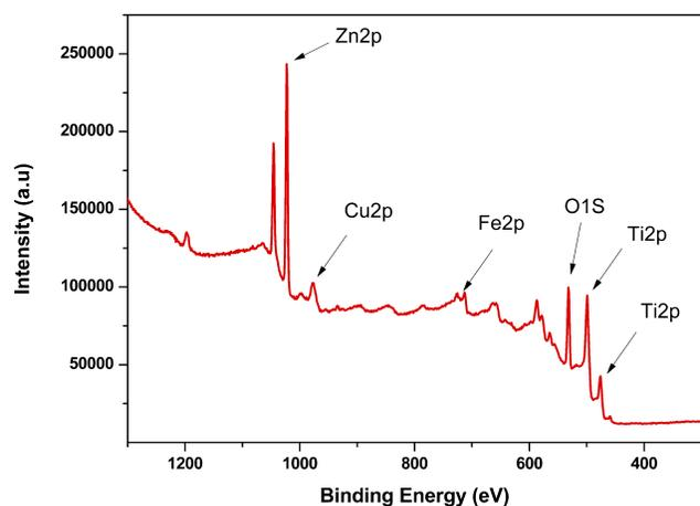
**Figure 2** XPS spectrum of titanate nanotubes/CuFe<sub>2</sub>O<sub>4</sub>/Zn-Fe MMO.
