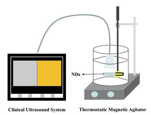
$\textbf{Figure I} \ \, \textbf{Setup to monitor the echogenicity of NDs as UCAs for ultrasound imaging}.$
