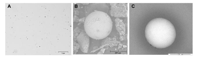
Figure 3 Morphology and structure of NDs. (A) The optical microscope (×1000) image (the scale bar represents 5 μm). (B) The SEM image (the scale bar represents 200 nm). (C) The TEM image (the scale bar represents 200 nm).
