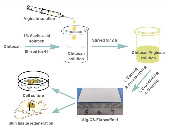
Figure I Schematic of preparation for fabrication of Alg-CS-Flu scaffolds.
