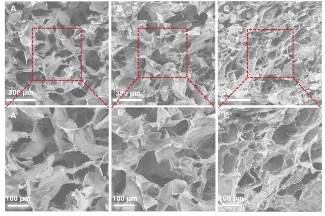
Figure 3 Cross-sectional SEM images of scaffolds: (A and A') Alg/CS scaffold; (B and B') Alg-CS scaffold; (C and C') Alg-CS-Flu scaffold.
