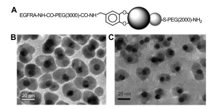
Figure 12 (A) Schematic illustration of surface functionalization of the Au–Fe<sub>3</sub>O<sub>4</sub> NPs. (B and C) TEM images of the 8–20 nm Au–Fe<sub>3</sub>O<sub>4</sub> particles before (B) and after (C) surface modification. Reprinted with permission from Xu C, Xie J, Ho D, et al. Au–Fe<sub>3</sub>O<sub>4</sub> dumbbell nanoparticles as dual-functional probes. Angew Chem Int Ed. 2008;47 (1):173–176.<sup>65</sup> Copyright © 2008 John Wiley and Sons.
