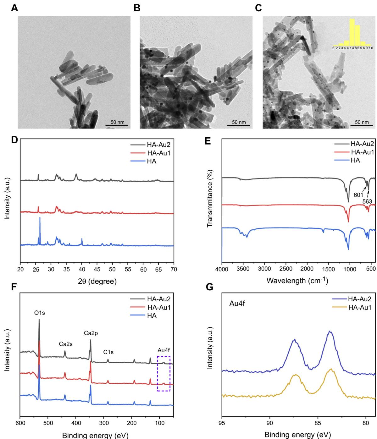
**Figure 1** TEM images of (A) HA, (B) HA-Au1, and (C) HA-Au2 (scale bar, 50 nm). (D) XRD, (E) FT-IR, (F) XPS analysis of HA, HA-Au1, and HA-Au2. (G) The high-resolution spectra of Au4f for HA-Au1 and HA-Au2.
