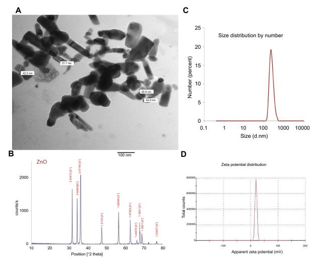
Figure I Characterization of ZnO-NPs (**A**) A representative micrograph of ZnO-NPs using TEM showing average particle size=40 nm, (**B**) XRD pattern of ZnO nanopowder showed peaks at 20=31.67°, 34.31°, 36.14°, 47.40°, 56.52°, 62.73°, 66.28°, 67.91°, 69.03° and 72.48°, (**C**) zeta potential of ZnO-NPs, (**D**) the hydrodynamic diameter of 100% ZnO-NPs using DLS.
