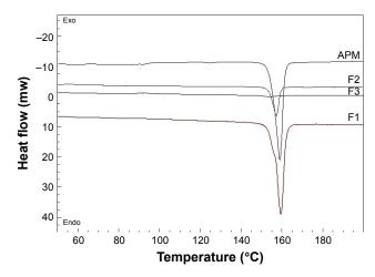
**Figure 2** DSC thermogram of APM and APM-loaded PLGA NPs (FI-F3). **Abbreviations:** APM, apremilast; DSC, differential scanning calorimetry; PLGA NPs, poly(D,L-lactide-coglycolide) nanoparticles.
