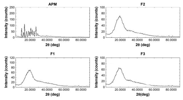
**Figure 3** Powder X-ray diffraction pattern of APM and APM-loaded PLGA NPs (FI-F3). **Abbreviations:** APM, apremilast; PLGA NPs, poly(D,L-lactide-coglycolide) nanoparticles.
