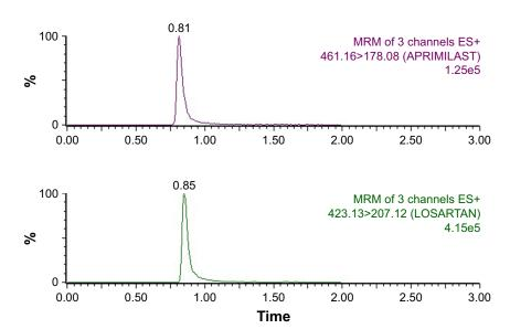
Figure 8 Representative MRM chromatogram of APM and IS in actual plasma sample at 1 hour after oral administration of APM (2 mg/kg). Abbreviations: APM, apremilast; IS, internal standard; MRM, multiple reaction monitoring.
