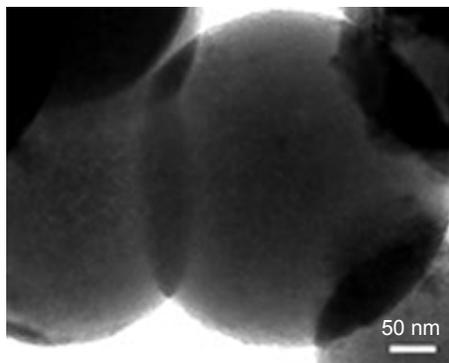
**Figure S1** TEM image of BG microspheres without hollow structure.
