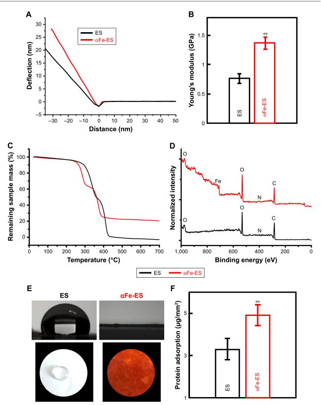
Figure 4 Physical and surface properties of the scaffolds (ES control and  $\alpha$ Fe-ES). (A) Representative deflection-distance curves of the electrospun scaffolds. (B) Young's modulus of ES and  $\alpha$ Fe-ES by nano indentation (n=4). (C) TGA results of the samples' weight loss during thermal treatment. (D) XPS spectra of the two groups. (E) Water contact angles of the two groups. (F) Measurements of protein adsorption (n=9). Note: \*\*P<0.01.
