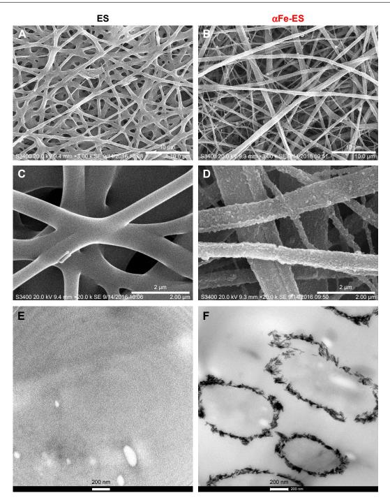
Figure 2 SEM (A–D) and TEM (E, F) images of the scaffolds: ES Control (A, C, E);  $\alpha$ Fe-ES (B, D, F). Note: The images present the morphology of the nano assemblies on the outer surface of the electrospun scaffolds. Abbreviations:  $\alpha$ FeNP, hydrophilic hematite nanoparticle;  $\alpha$ Fe-ES,  $\alpha$ FeNPs-assembled electrospun scaffold; ES, untreated electrospun scaffold; SEM, scanning electron microscopy; TEM, transmission electron microscopy.
