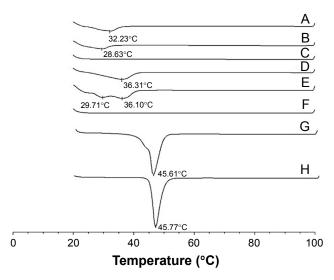
**Figure 4** Differential scanning calorimetry curve of the mixtures of orlistat, Solutol HS15, and Lauroglycol 90; SSPH6 (**A**), SSPL6 (**B**), LSP11 (**C**), NSP6 (**D**), binary mixture of orlistat and Solutol HS15 (50:50, w/w) (**E**), Solutol HS15 (**F**), treated orlistat (**G**), or raw orlistat (**H**).
