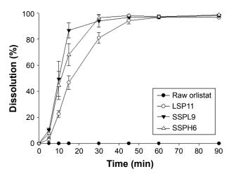
**Figure 7** Dissolution profiles of raw orlistat, LSP11, SSPL9, or SSPH6 at pH 1.2 (n=4). **Abbreviations:** LSP, liquid-SNEDDS preconcentrate; SNEDDS, self-nanoemulsifying drug delivery system; SSPH, solid SNEDDS preconcentrate of a high melting temperature; SSPL, solid SNEDDS preconcentrate of a low melting temperature.
