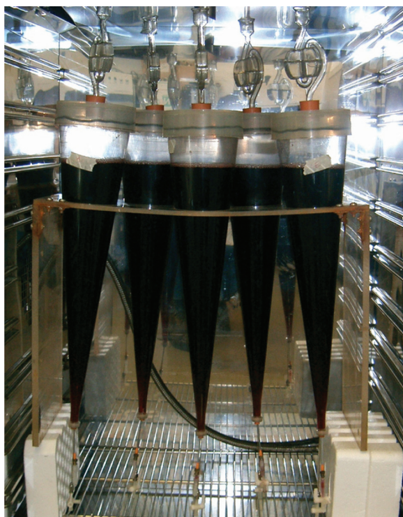
Figure 6 Imhoff conical vessels used in small-scale wine fermentation. Wine yeast strains were grown in graduated conical vessels (1 L, cone angle 74°) made of polycarbonate and closed with fermentation locks. Cones were washed previously with nitric acid, ddH 2 O, EDTA (as described in Materials and methods) and filled with grape juice. Yeast cells were inoculated at initial cell density of 12 \times 10^6 cells/mL and fermentation was carried out at 25 °C for five days.
