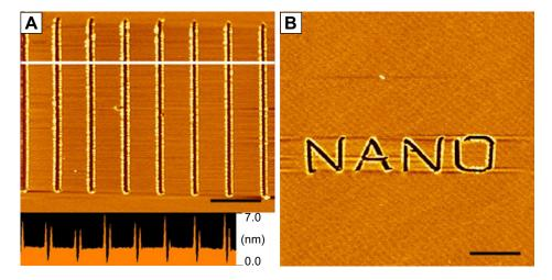
Figure 13 Nanopatterns generated by AFM nanolithography on a peptide self-assembled monolayer on mica surface.
