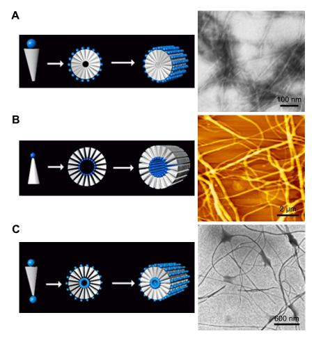
Figure 6 Self-assembly of amphiphilic peptides with different geometrical shapes.
