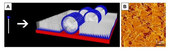
Figure 4 Monolayer film formed by surfactant-like peptide A6K on mica surface.
