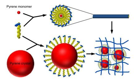
$\textbf{Figure II} \ \, \textbf{Two mechanisms for the encapsulation of hydrophobic pyrene by A6K}.$
