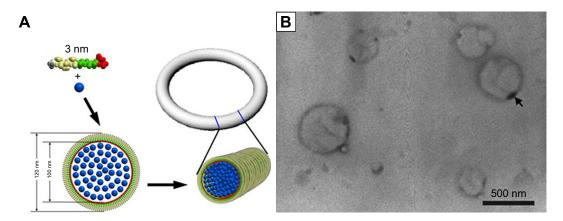
Figure 12 Copper particle nanorings induced by surfactant-like peptide.
