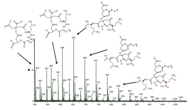
Figure 3 Liquid chromatography-mass spectroscopy of glutamine conjugated to dendrimer-G,
