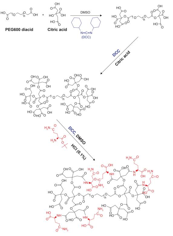
**Scheme I** The preparation routes of dendrimer- $G_2$  and glutamine conjugation. **Abbreviations:** DCC, N, N'-dicyclohexylcarbodiimide; DMSO, dimethyl sulfoxide.
