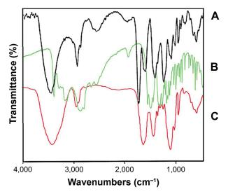
Figure 1 Fourier transform infrared spectrum of (A) dendrimer-G<sub>2</sub>, (B) glutamine, and (C) dendrimer–glutamine.
