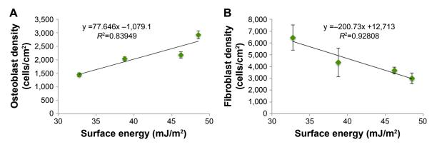
Figure 12 (A) Osteoblast and (B) fibroblast cell density (after 4 hours of culture) was directly proportional to the surface energy on Ti controls and Ti-TiO<sub>2</sub> samples. Error bars represent SD.
