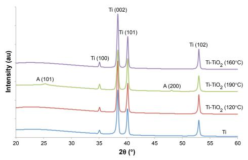
**Figure 3** XRD patterns of the Ti samples with different  $TiO_2$  coatings. **Abbreviations:** A, anatase; Ti, titanium;  $TiO_2$ , titanium dioxide; XRD, X-ray diffraction.
