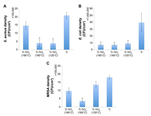
Figure 4 (A) S. aureus, (B) E. coli, and (C) MRSA growth on Ti samples with different  $TiO_2$  coatings after 24 hours of culture. Data represent mean  $\pm$  SD, N=3. \*p<0.05 compared with Ti control (labeled as Ti).
