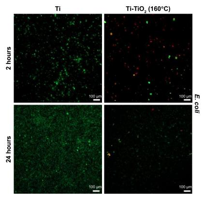
Figure 6 Fluorescent micrographs of *E. coli* cultured for 2 hours and 24 hours on Ti and Ti-TiO $_2$  (160°C) samples. SYTO $^8$  9 and propidium iodide were used to stain live (green) and dead (red) bacteria cells, respectively. Scale bars are 100  $\mu$ m. **Abbreviations:** *E. coli*, *Escherichia coli*; Ti, titanium; TiO $_2$ , titanium dioxide.
