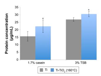
**Figure 8** The amount of adsorbed casein protein and total proteins on sample surfaces after 24 hours of culture in a 1.7% casein solution and 3% TSB medium. Data represent mean  $\pm$  SD, N=3. \*p<0.05 compared with Ti control (labeled as Ti) in the same tested solution.
