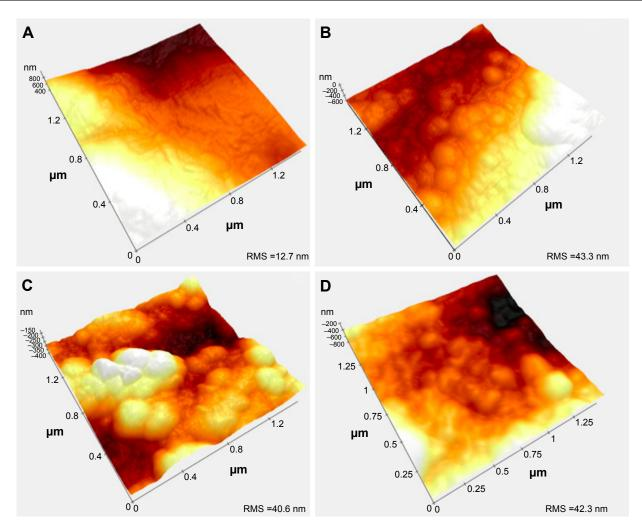
Figure 2 AFM images and RMS roughness values (in nm) of (A) Ti control, (B) Ti-TiO<sub>2</sub> (190°C), (C) Ti-TiO<sub>2</sub> (160°C), and (D) Ti-TiO<sub>2</sub> (120°C). Abbreviations: RMS, root-mean-square; Ti, titanium; TiO<sub>2</sub>, titanium dioxide; AFM, atomic force microscopy.
