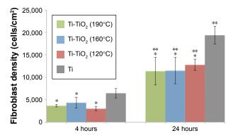
**Figure 11** Fibroblast adhesion and growth on Ti and Ti-TiO $_2$  samples. Data represent mean  $\pm$  SD. \*p<0.05 compared with Ti control at the same time period, \*\*p<0.05 compared with the same sample (4 hours).
