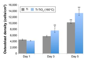
**Figure 10** Osteoblast proliferation on Ti and Ti-TiO $_2$  (160°C) samples. Data represent mean  $\pm$  SD. N=3. \*p<0.05 compared with Ti at the same time period, \*\*p<0.05 compared with the same sample (Day I).
