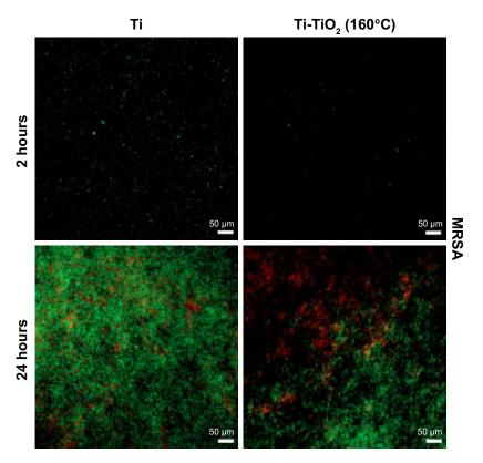
Figure 7 Fluorescent micrographs of MRSA cultured for 2 hours and 24 hours on Ti and Ti-TiO<sub>2</sub> (160°C) samples. SYTO® 9 and propidium iodide were used to stain live (green) and dead (red) bacteria cells, respectively. Scale bars are 50 μm. **Abbreviations:** MRSA, methicillin-resistant *Staphylococcus aureus*; Ti, titanium; TiO<sub>3</sub>, titanium dioxide.
