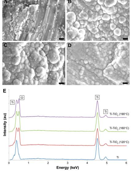
Figure I SEM images of (A) Ti control, (B) Ti-TiO<sub>2</sub> (190°C), (C) Ti-TiO<sub>2</sub> (160°C), and (D) Ti-TiO<sub>2</sub> (120°C) and (E) EDAX spectra of Ti samples. Scale bars are 200 nm. Abbreviations: O, oxygen; SEM, scanning electron microscopy; Ti, titanium; TiO<sub>2</sub>, titanium dioxide.
