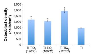
**Figure 9** Osteoblast adhesion on Ti samples with different  $\text{TiO}_2$  coatings after 4 hours of culture. Data represent mean  $\pm$  SD, N=3. \*p<0.05 compared with Ti control (labeled as Ti).
