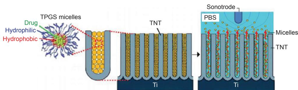
**Figure 9** Schematic illustration of ultrasound-stimulated DD based on TNT implants and polymeric micelles as drug carriers. Reprinted from *Int J Pharm*, 443, Aw MS, Losic D. Ultrasound enhanced release of therapeutics from drug-releasing implants based on titania nanotube arrays, 154–162.<sup>97</sup> Copyright (2013), with permission from Elsevier. **Abbreviations:** DD, drug delivery; PBS, phosphate-buffered saline; TNT, titania nanotube.
