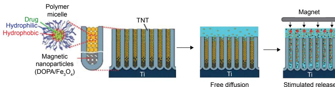
**Figure 8** Schematic representation of the magnetic stimuli-responsive drug release from TNTs which integrates polymer micelles as drug carriers incorporated with poorly soluble drugs and magnetic nanoparticles loaded at the bottom of the nanotubular structures.
