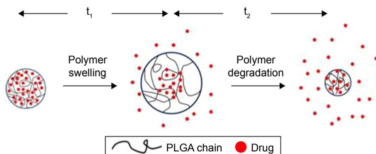
**Figure 4** Schematic diagram explaining pH-dependent drug release shape.
