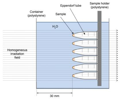
Figure 1 Sketch of the sample irradiation geometry.
