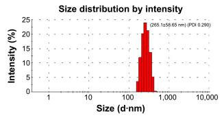
**Figure 3** The size distribution of the novel NP-siRNA liposomes. **Notes:** The size and the zeta potential of the novel NP-siRNA liposomes were measured using a Malvern Zeta Nanosizer ZS 90. The peak size of the novel NP-siRNA liposomes was 265. I nm with a PDI of 0.290 and zeta potential was 31.8 mV. **Abbreviations:** NP, nanoparticle; PDI, polydispersity index; siRNA, small interfering RNA.
