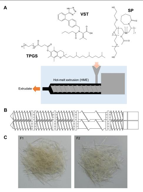
Figure I Preparation of VST-loaded SD formulations.
