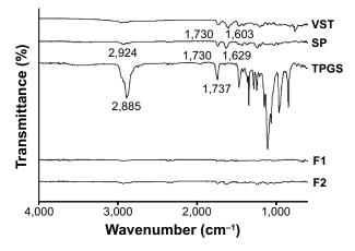
Figure 2 FT-IR spectra of VST, SP, TPGS, FI, and F2. Abbreviations: FI and F2, solid dispersion formulations used in this study; FT-IR, Fourier-transform infrared; SP, Soluplus; TPGS, D-alpha-tocopherol polyethylene glycol 1000 succinate; VST, valsartan.
