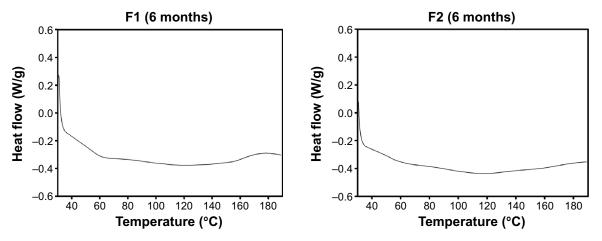
Figure S1 DSC thermograms of F1 (6 months) and F2 (6 months). Abbreviations: DSC, differential scanning calorimetry; F1 and F2, solid dispersion formulations used in this study.
