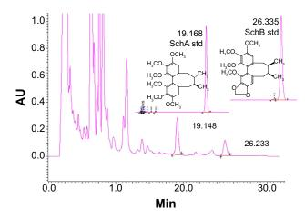
**Figure 1** The chromatograms of schisandrin (Sch) A and SchB, two major active components of *Schisandra chinensis* extract under high-performance liquid chromatography analysis. The column was eluted using  $H_2O$ :methanol (v/v, 30:70) at a flow rate of 1.0 mL/minute for 35 minutes. The absorbance at 254 nm was monitored.
