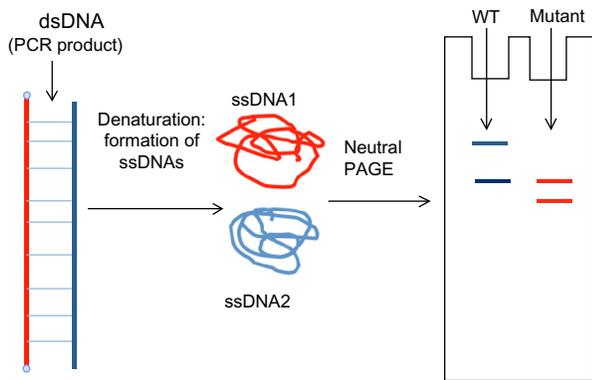
**Figure 6** The single-strand conformation polymorphism process. After denaturation of the polymerase chain reaction (PCR) product, the conformation of single-stranded DNA (ssDNA) could be different, resulting in altered mobility in polyacrylamide gel. **Abbreviations:** dsDNA, double-strand DNA; PAGE, polyacrylamide gel electrophoresis; WT, wild type.
