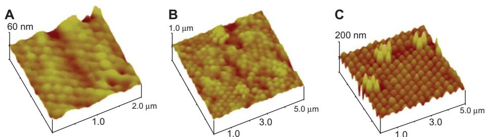
**Figure 1** Atomic force microscopy images of the poly(lactic-co-glycolic acid) surfaces synthesized using a template covered with polystyrene nanobeads. The dimensions of the polystyrene nanobeads were: (A) 190 nm, (B) 300 nm, and (C) 400 nm. Spherical surface features were effectively transferred to the poly(lactic-co-glycolic acid) surfaces, and ordered surface features were observed.
