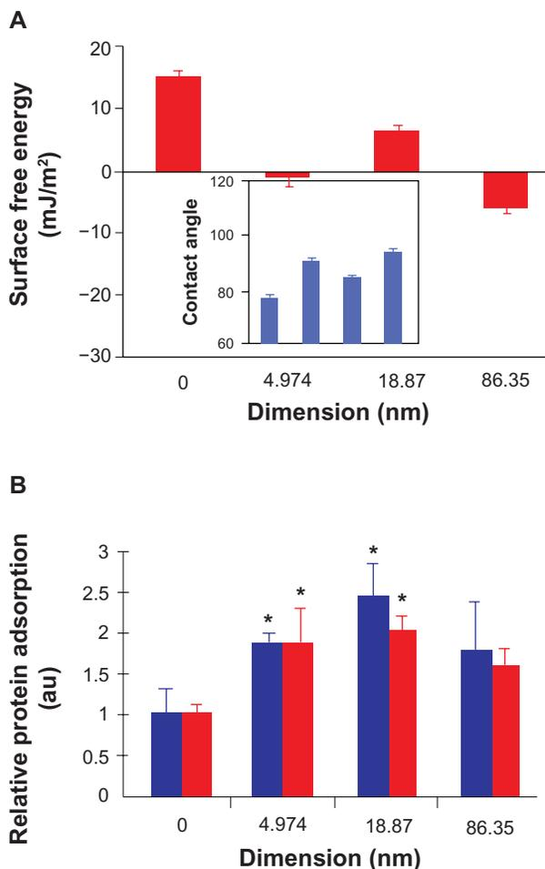
**Figure 2** The effect of the change in the poly(lactic-co-glycolic acid) surface feature size on (A) surface energy (red) and water contact angles (blue), and (B) relative collagen type IV (blue or left) and fibronectin (red or right) adsorption. Surface energy and water contact angle results are significantly ( $P < 0.05$ ) different between all data points. Values are mean  $\pm$  standard error of the mean. \* $P < 0.05$  compared with control surfaces.
