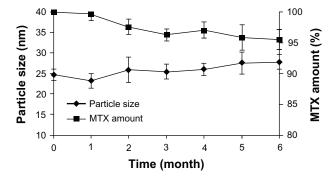
**Figure 4** Particle sizes and MTX amounts of lyophilized mixed micelles kept at 4°C as a function of time.
