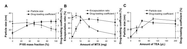
Figure I Particle size and drug-loading coefficient of mixed micelles with different P105 mass fraction (**A**); drug-loading coefficient and encapsulation ratio of mixed micelles as a function of amount of MTX loading (**B**); particle size and drug-loading coefficient of mixed micelles as a function of TEA volume (**C**). Note: Values are means  $\pm$  standard deviation (n = 3). Abbreviations: MTX, methotrexate; TEA, triethylamine.
