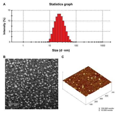
Figure 2 Particle size and size distribution of PF-MTX measured by dynamic light scattering (**A**); transmission electron microscopy image of PF-MTX, the bar is 100 nm (**B**); atomic force microscopy image of PF-MTX (**C**). **Abbreviation:** PF-MTX, methotrexate loaded P105/F127 mixed micelles.
