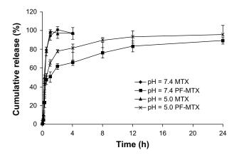
Figure 5 Release profiles of MTX from mixed micelles in PBS (pH 7.4) or acetate buffer (pH 5.0) medium at  $37^{\circ}$ C.
