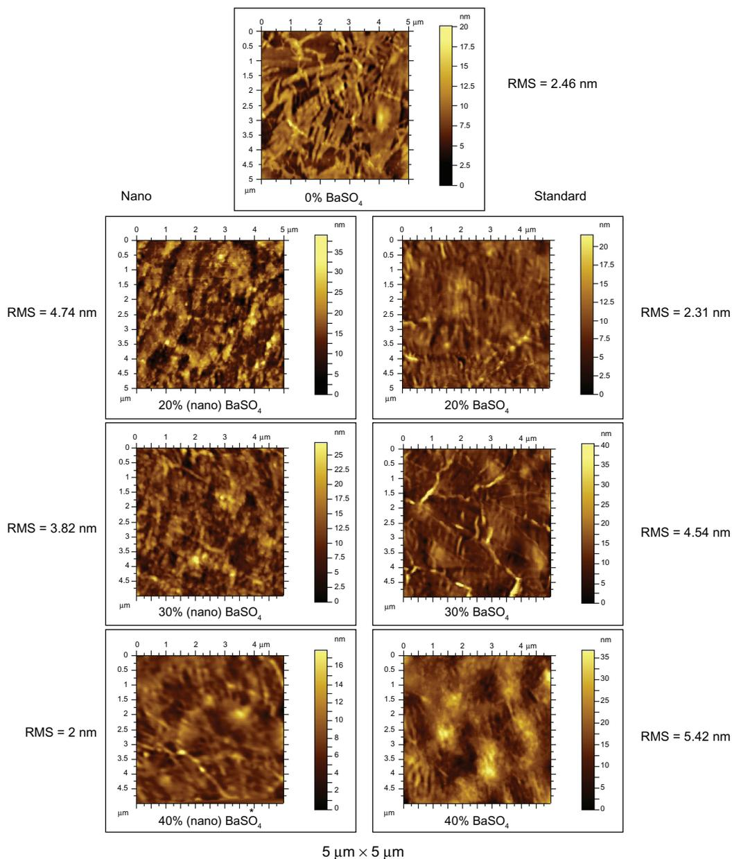
**Figure 3** AFM 5 μm × 5 μm scan areas on polymer samples.
