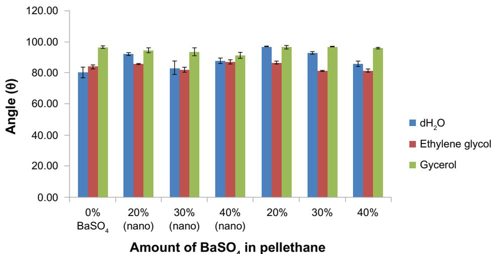
**Figure 1** Contact angle measurements on pellethane samples.
