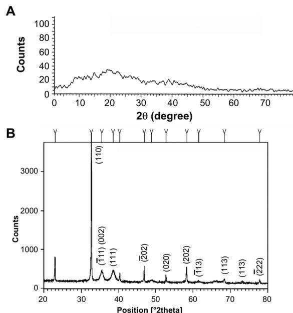
**Figure 2** XRD pattern of synthesized CuO nanoparticles. XRD pattern of (A) GK and (B) CuO nanoparticles, indicating the amorphous nature of GK and the crystalline nature with different planes of synthesized CuO nanoparticles.
