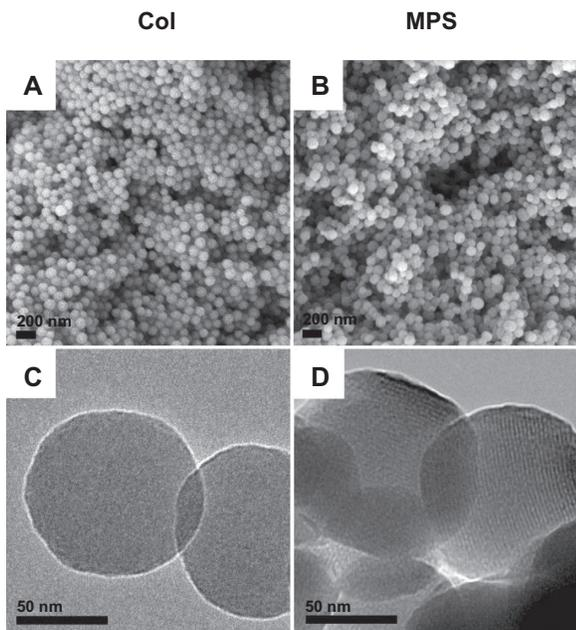
**Figure 1** (A and B) FE-SEM and (C and D) TEM images of Col and MPS NPs. **Abbreviations:** FE-SEM, field emission scanning electron microscopy; TEM, transmission electron microscopy; MPS, mesoporous silica; Col, colloidal silica; NPs, nanoparticles.
