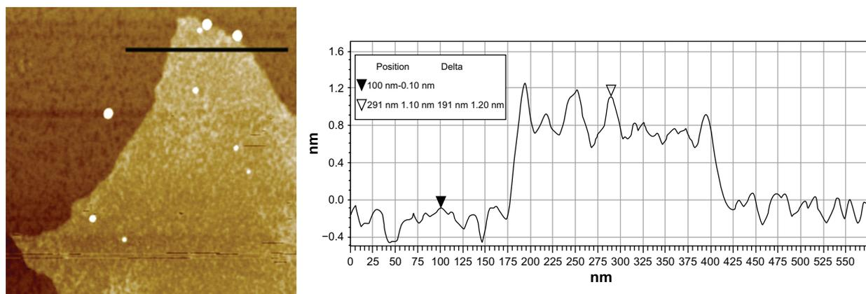
**Figure 2** Atomic force microscopy measurement of graphene oxide (scan area:  $1 \mu\text{m} \times 1 \mu\text{m}$ ). Tapping mode atomic force microscopy image of single-layer graphene oxide (KS-20) with corresponding height cross-sectional profile with an average thickness of 1.2 nm. The sample was spin-coated on a freshly cleaved mica substrate.
