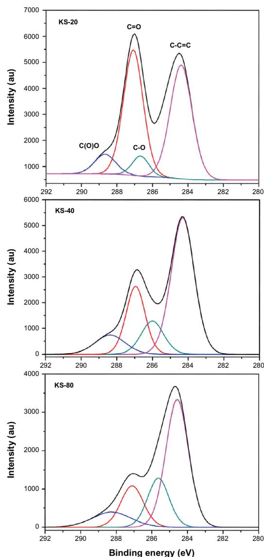
**Figure 4** X-ray photoelectron spectrometry analysis of graphene oxide with different degrees of oxidation illustrating the deconvoluted X-ray photoelectron spectra in the C1s peak region for the KS-20, KS-40, and KS-80 samples.
