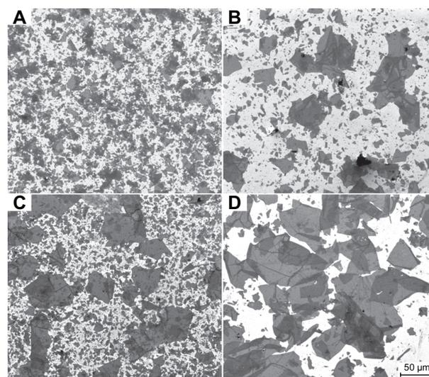
**Figure 1** Field emission scanning electron microscopy micrographs of graphene oxide prepared in (A) KS-80, (B) KS-40, and (C) KS-20 after 3 days of oxidation and (D) nonsonicated KS-20. All the micrographs were taken at the same magnification.
