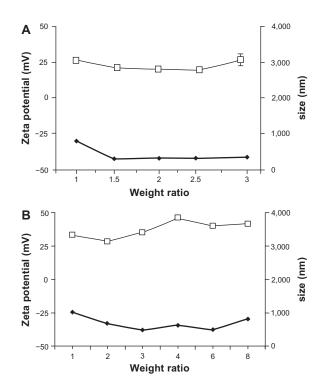
Figure 2 Zeta potential (□) and particle size (♦) at varying weight ratios of complexes formulated with (A) poly-L-arginine (PLA)/DNA and (B) PLA-coated liposomes (PCL)/DNA.
