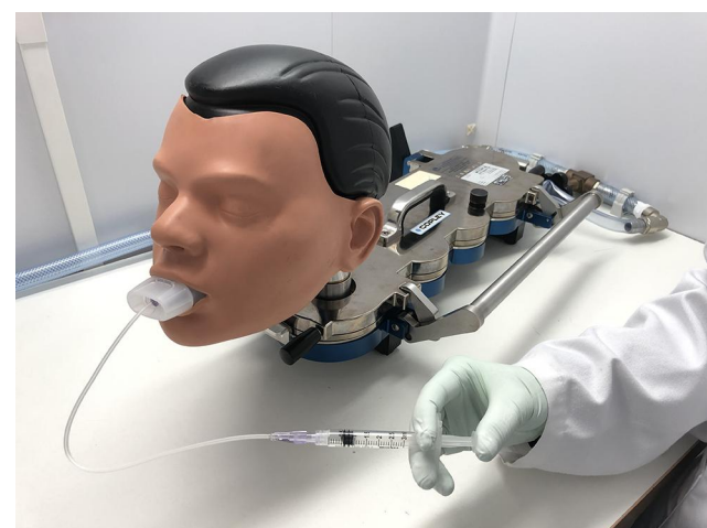
Figure 2 The Trachospray device connected to an Alberta Idealized Throat and a Next Generation Impactor.
