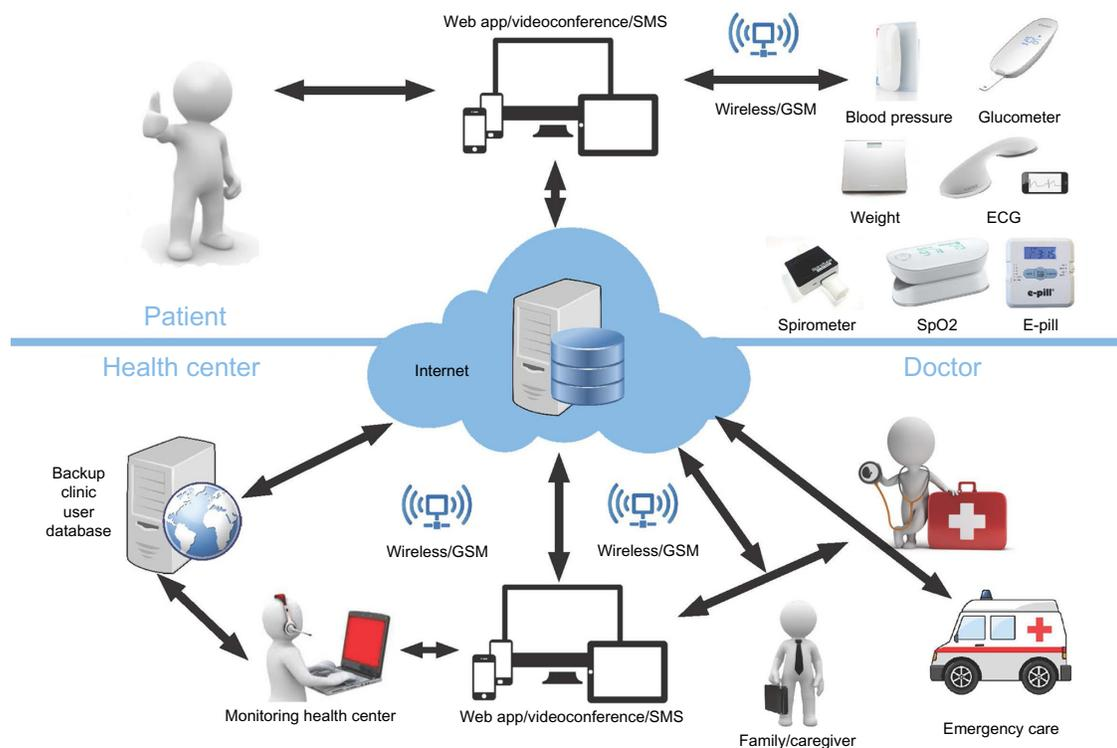
**Figure 1** Scheme of a home telecare system.
