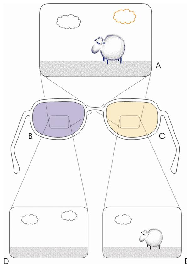
**Figure 1** A diagram of the anaglyphic system for amblyopia treatment. The display (A) consists of elements that, based on color, may be visible by one or both eyes. The filter for the unaffected eye (B) filters out main moving elements (D), while the filter of the amblyopic eye (C) allows for the eye to see the main elements and may or may not filter out less significant features (E).
