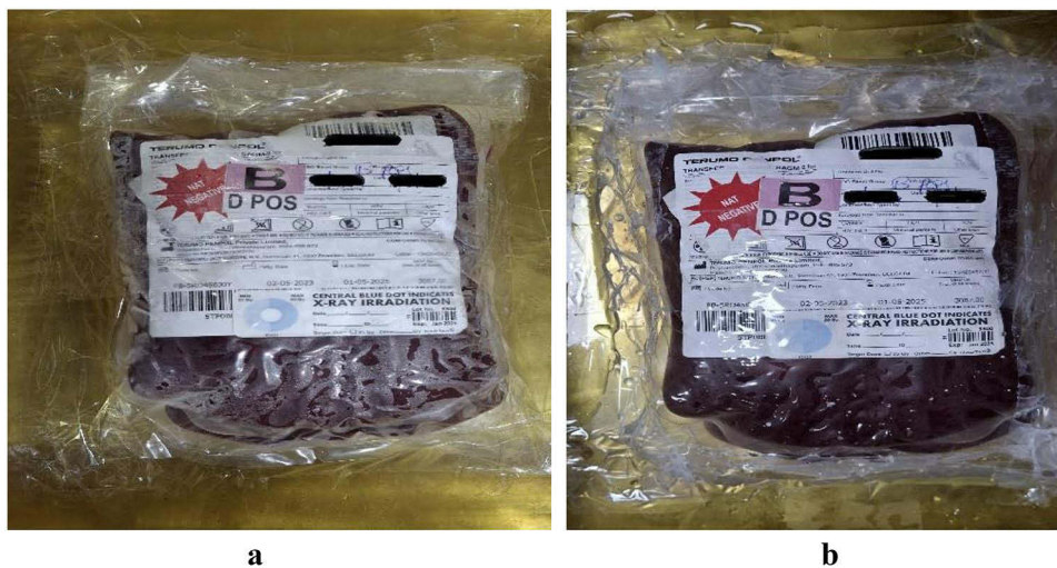
Figure 4 Film indicator before (a) and after (b) irradiation (25 Gy).
