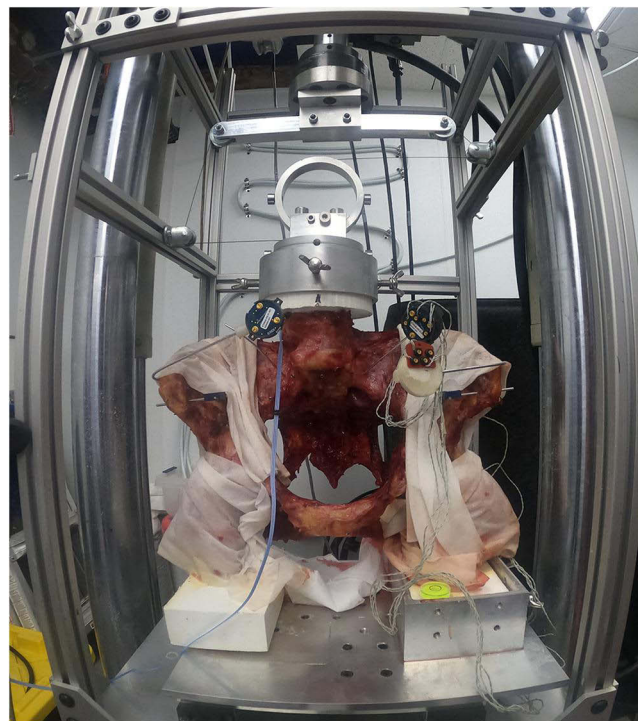
Figure 4 Test Setup Of The Left Side In An Intact Pelvis Under Left (Ipsi) Lateral Bending Moment Load.
