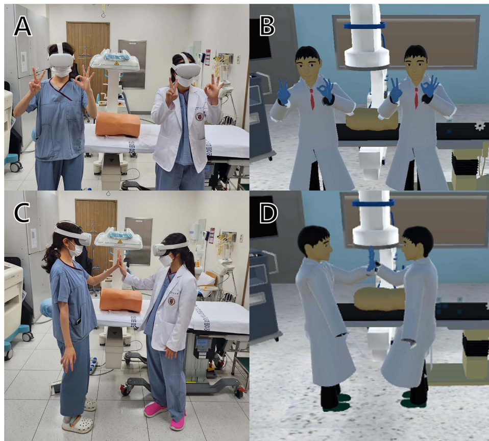
Figure 1 Networked virtual simulator with postural and spatial awareness. (A) Two trainees wearing the devices making hand gestures. (B) Avatars in the virtual space mirroring the hand gestures. (C) Hand-to-hand testing of spatial alignment in an actual procedure room. (D) Note the successful spatial matching between the avatars connected to the virtual space through the network.
