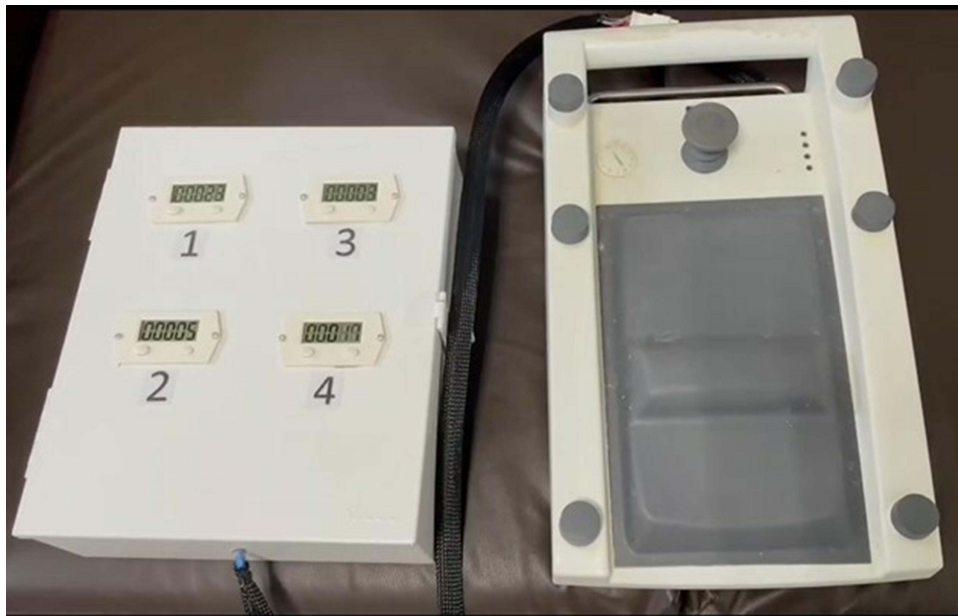
Figure 1 Counter connected to the microscope footswitch.
