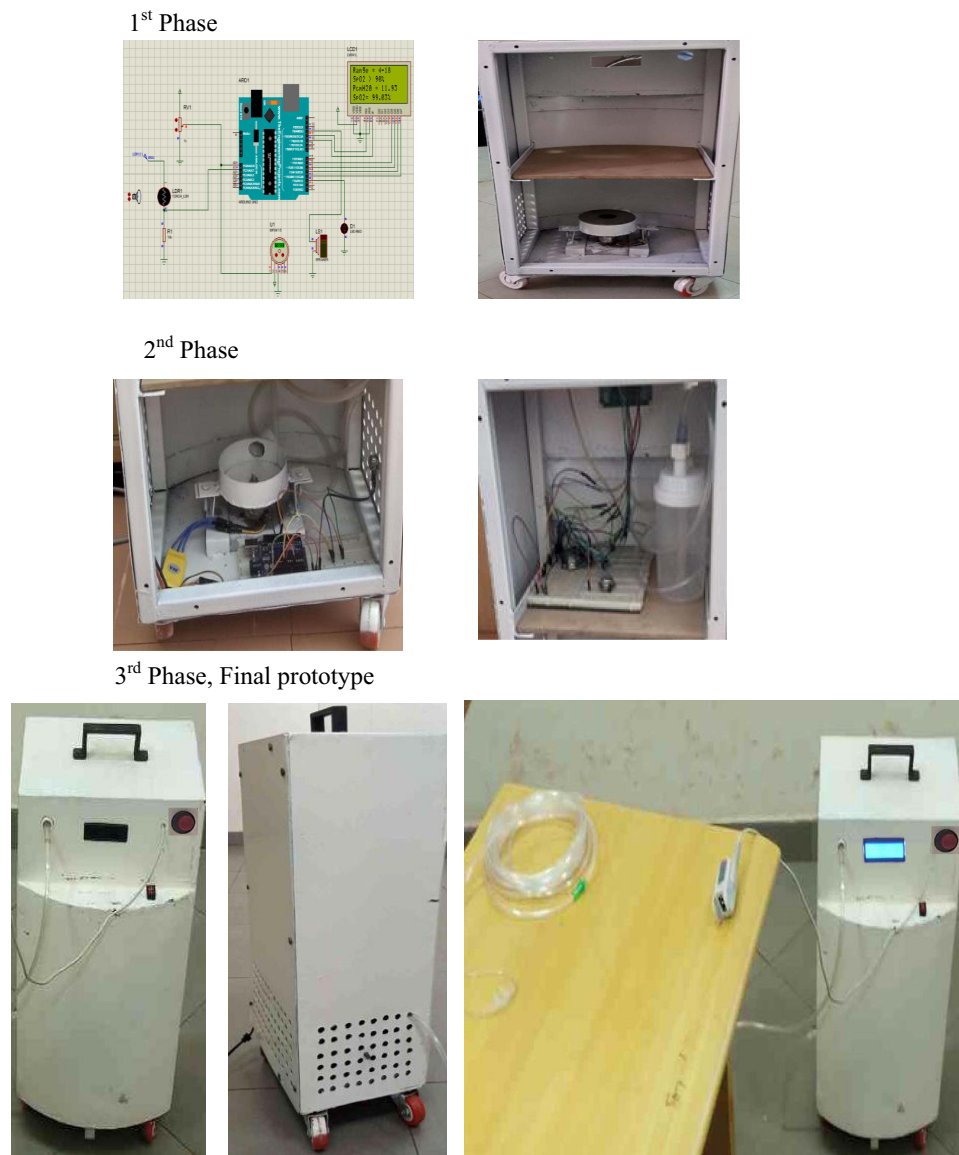
Figure 7 The overall development process of the prototype (1 st Phase: Design and simulating on computer aided design software, Functional test based on simulation parameters and made appropriate design revision. 2 nd Phase: Construction of centrifugal fan including Power supply, Controlling unit including humidifier, Constructing all components of the design. 3 rd Phase: Images of final prototype from different position).
