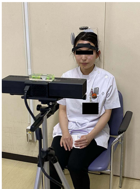
Figure 2 Photograph showing simultaneous measurement of the head posture with KSSM and CROM3 The Kinect v2 was fixed at the participant's eye level while sitting at a distance of 1.0 m from the device. CROM3 was fitted on the back of the participant's heads to increase the accurate face recognition without any interference caused by the front indicator of the CROM3 device. We have obtained individual permission to publish photograph of the subject in the journal.
