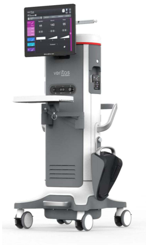
Figure 1 The VERITAS Vision System. The system has two procedure packs with an advanced tubing system (small bore and dual durometer aspiration tubing). The system also has an advanced infusion pack with gas forced infusion functionality and updated venting algorithm. The 19-inch monitor has 15° of tilt and 80° of side-to-side rotation for ease of viewing. The user interface has been enhanced for ease of access to menus and case information. There is a flat tray with tube holders for easy cord management.
