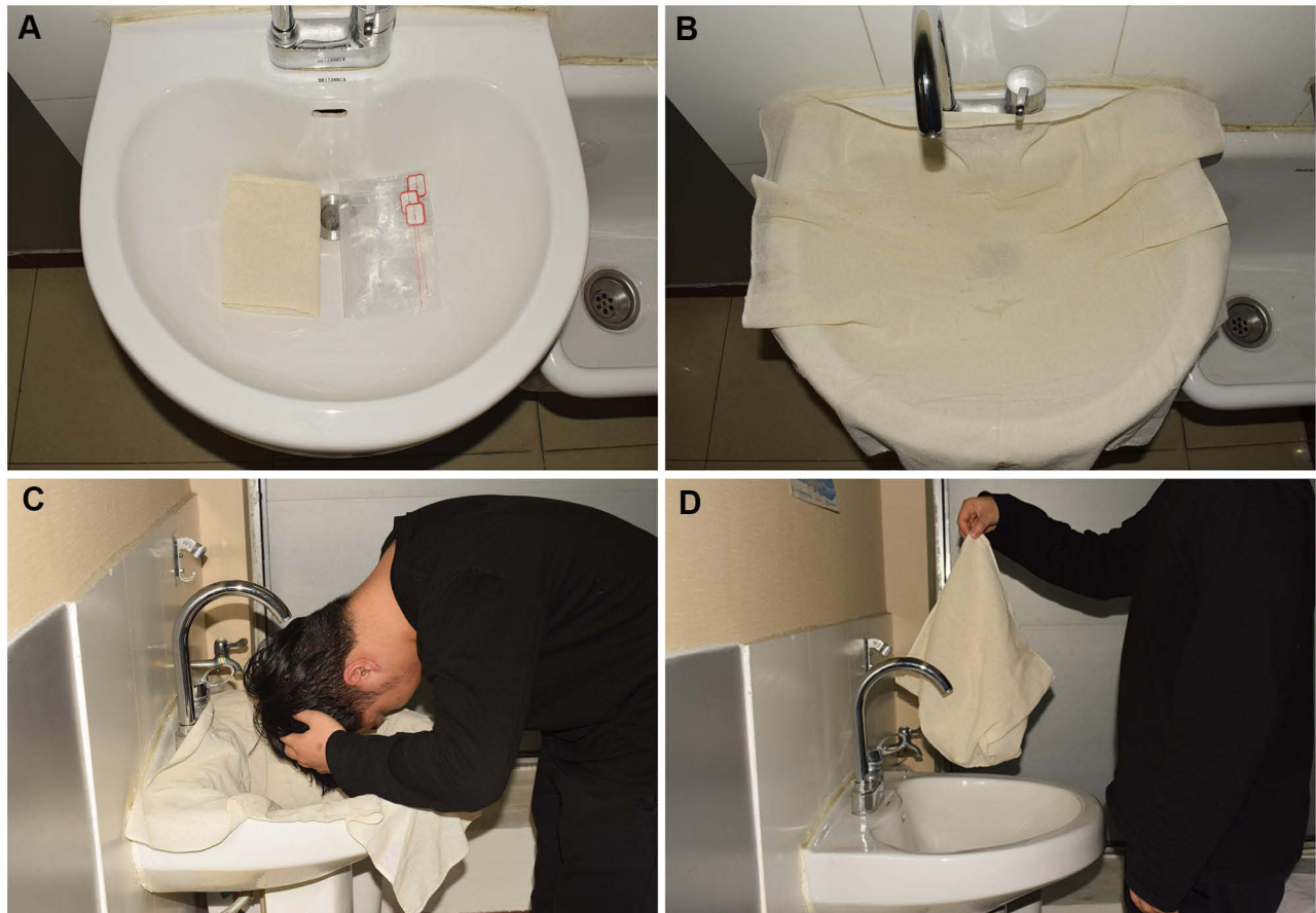
Figure 1 The demonstration of refined wash test procedure. (A) The supplies necessary for the test. (B-D) The subjects were asked to spread a piece of filter cloth with light color over the sink and shampoo with flowing water above the cloth. They washed their hair once, from hair roots to tips, rinsed the hairs gently and kept the water draining away directly to the sewer.
