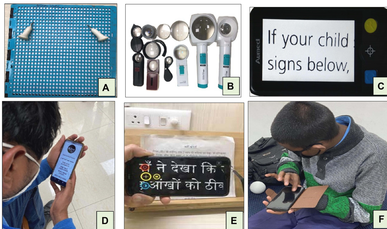
Figure 4 Assistive technology for visual impairment (First row: traditional products: (A) Braille slate and stylus, (B) optical magnifiers, (C) video magnifiers; second row: smartphones accessible apps: (D) Kibo, (E) Visor, (F) operating TalkBack.
