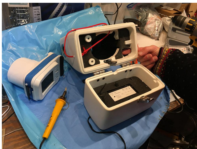
Figure 2 Finger cut-out in the back section of Kaleidos battery case allowing trigger activation of the 2WIN photoscreener.
